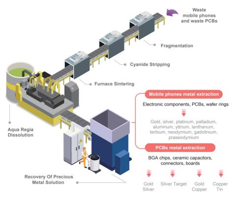
Figure7. Common E-waste Recycling – Metal Extraction Process
